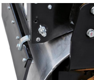
Wear-resistant scraper can be lift and fixed during transportation
