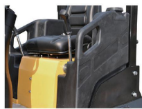
Emulsified liquid tank
